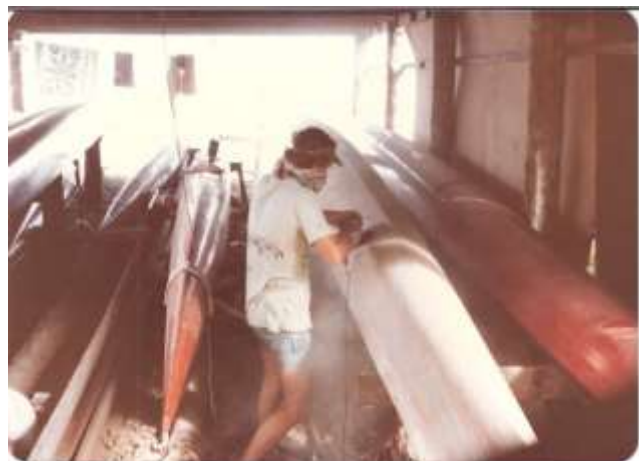
Shaping outrigger canoes. These canoes were made of Falcatta trees (Albizia).
