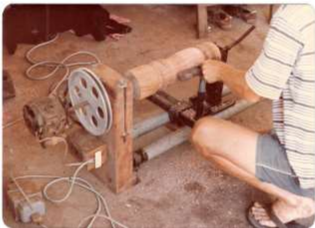
I made this lathe using a washing machine motor.
