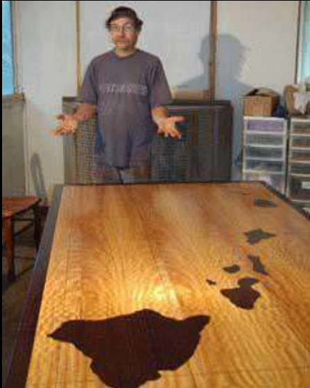
Mango Office Unit with Black Wenge Wood accents. For the desk, I took a chart of the Hawaiian Islands, made longitude and latitude lines with inlayed Wenge wood, and then inlayed the islands so that the desktop is an accurate chart of the Hawaiian Islands.
